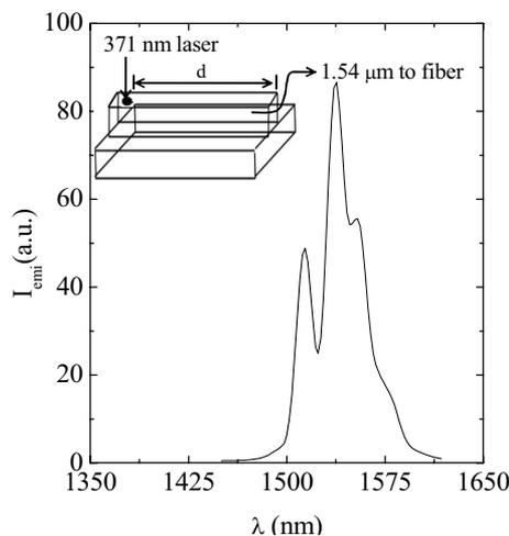
FIG. 2. PL spectra of Er-doped GaN waveguide amplifier taken from the end facet of the waveguide when the other end is illuminated by a 371 nm nitride laser.  $1.54 \mu\text{m}$  emission was generated at the laser excitation spot within the core of the waveguide and guided to the end facet of the waveguide. The inset shows the optical loss measurement setup.
