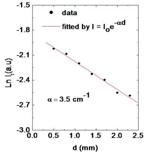
FIG. 3. (Color online) Plot of  $1.54 \mu\text{m}$  peak intensity as a function of laser excitation spot distance,  $d$ . The slope of the plot gives the optical loss, which is about  $3.5 \text{ cm}^{-1}$ .
