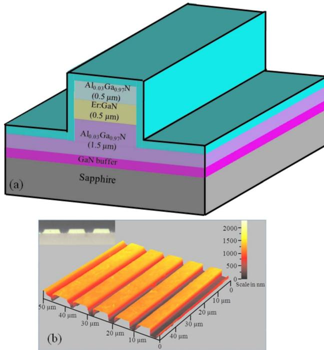
FIG. 1. (Color online) (a) Schematic layer structure of fabricated strip Er-doped GaN waveguide amplifier, which utilizes GaN:Er as optical gain medium with  $\text{Al}_{0.03}\text{Ga}_{0.97}\text{N}$  as top and bottom cladding layers, (b) atomic force microscopy image of fabricated devices. The inset shows the optical microscopy image of waveguide facets prepared by mechanical polishing.
